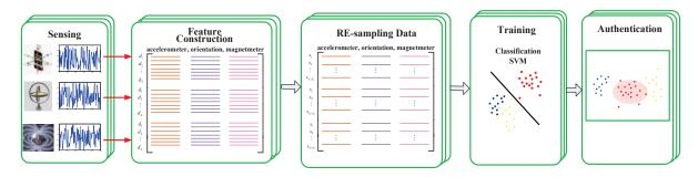
Figure 1: In our method, we first construct a vector at each time by using sensors' data (In experiment, we use 9 values from the accelerometer, magnetometer and orientation sensor in a smartphone.) After that, we re-sample the data collected from the sensors in a smartphone. Then, we train the re-sampled data with the SVM technique to get a user's profile. Based on the user's profile, we can do the implicit authentication.
